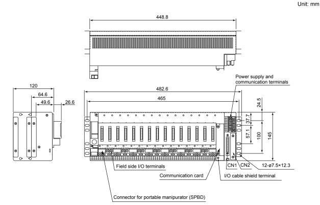
Note A mounting method is limited to horizontal installation in 19 inch rack of the EIA/JIS-standard.
